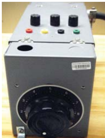
VARIAC ,SHOWING FUSES [WITHOUT FUSE- STATUS INDICATOR BOX]
