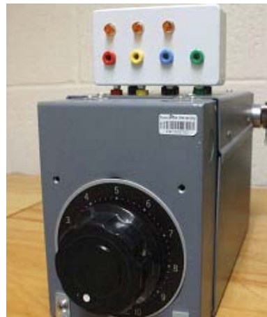
VARIAC ,[WITH FUSE-STATUS INDICATOR BOX MOUNTED]
